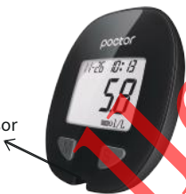
Figure 5 Position Diagram of Glucometer Temperature Sensor
